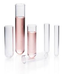
Note: Centrifuge tubes must be filled at least 80% for proper performance.
