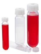
Note: Must be filled to 100% of total capacity for centrifugation.
