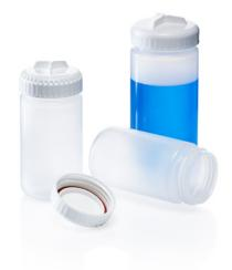
Note: For proper performance bottles must be filled to 80% of total capacity
