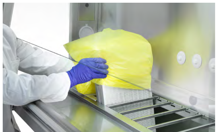
New unique sealing system simplifies installation and testing.
